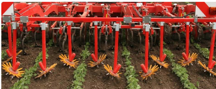
Picture 1: Combination of finger weeder and duck-foot tines in soy. Picture 2: Finger weeder at work within the row. (Pictures: Goran Malidza, Institute of Field and Vegetable Crops, Novi Sad).
